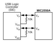
Figure 11. MIC2550A Interface to Non-multiplexed Data Bus
