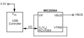
Figure 9. I/O Interface Using 3.3V
