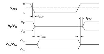
Figure 1. Enable and Disable Times
